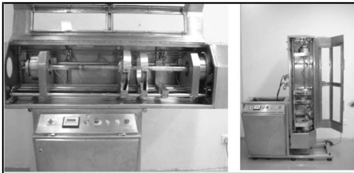
Indigenously developed zone refining unit
